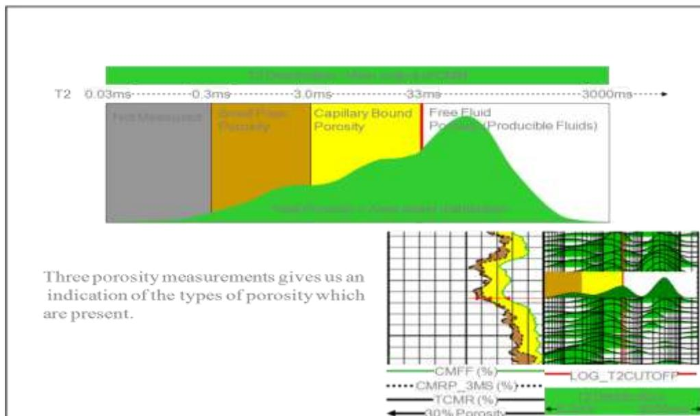
Fig. 4: The Porosity types according to  $T_2$  distribution cutoff.
