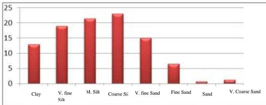
**Fig. 10:** Pore size distribution over the interval 9920' to 9948' of w. Al Khilala-1
