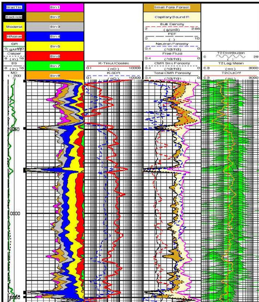
**Fig.7:** Bin porosity display over interval 9920' – 10,050' for W. Al Khiala-1 Well.
