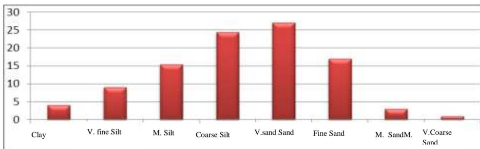
**Fig. 11:** Pore size distribution over the interval 9950' to 10,050' of W. Al Khilala-1 Well.
