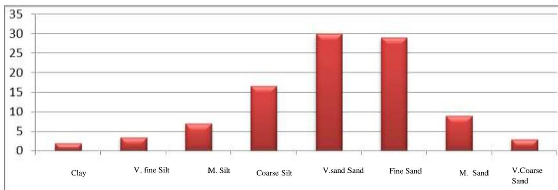
Fig. 13: Pore size distribution over the interval 9930' to 9964' of W. Al Khilala-2 well.
