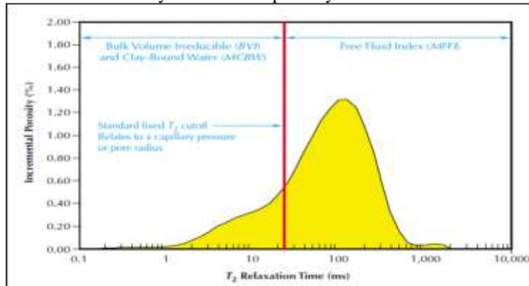
Fig. 6: The Standard fixed T2 cutoff to differentiate between CBW, BVI and FFI [21].
