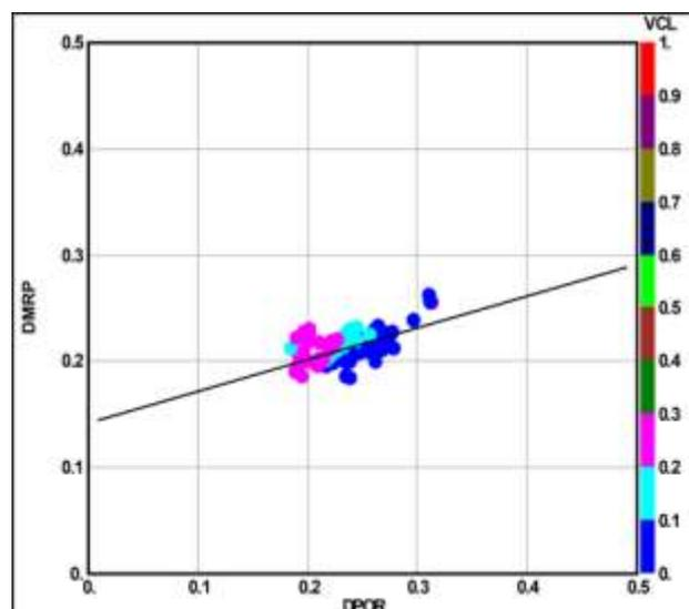
Fig. 5: The relation between density derived total porosity and DMRP of well W. Al Khilala-5well.
